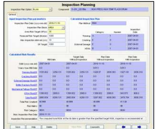
This plot shows the calculated damage progression over time, and “time stamped” date when the acceptable risk target will be reached. A recommended inspection plan is then generated based on the percentage of total risk by each individual damage mechanism.
