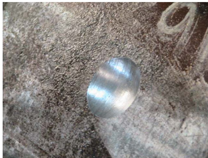
OD Sample from a 30 inch NPS C-1/2Mo Header
